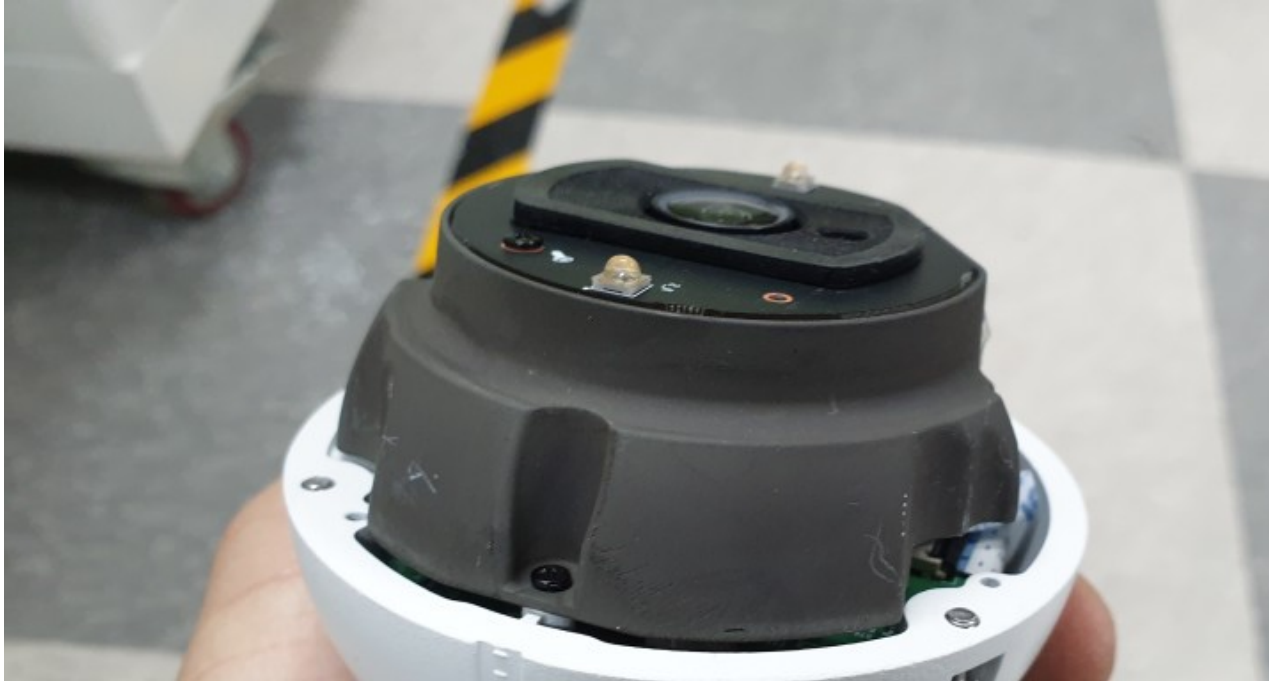
< Photo 12 > The second characteristic numeral test
