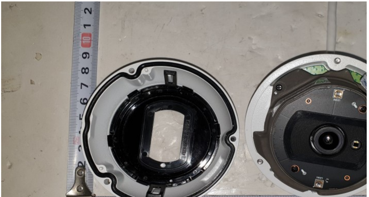
< Photo 12 > The second characteristic numeral test
