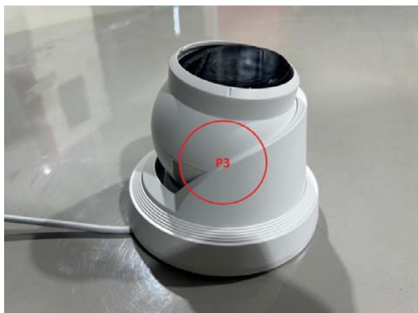
Check the hit area the test_4
