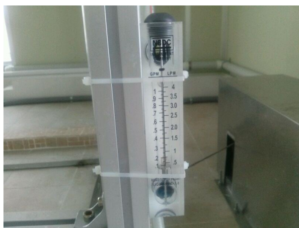
Water flow meter with Drip box
