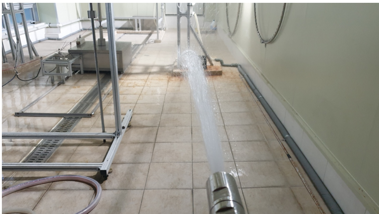
< Photo 4 > The second characteristic numeral test
