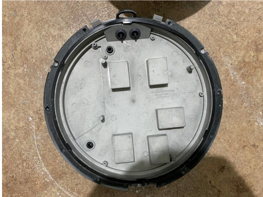
< Photo 8 > The second characteristic numeral test
