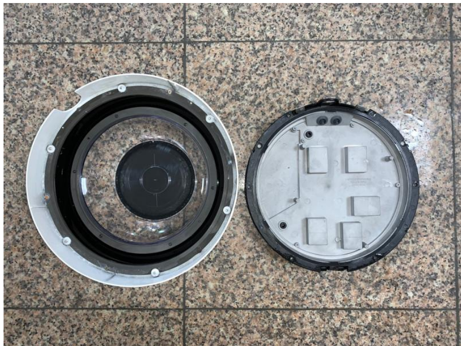
< Photo 8 > The second characteristic numeral test
