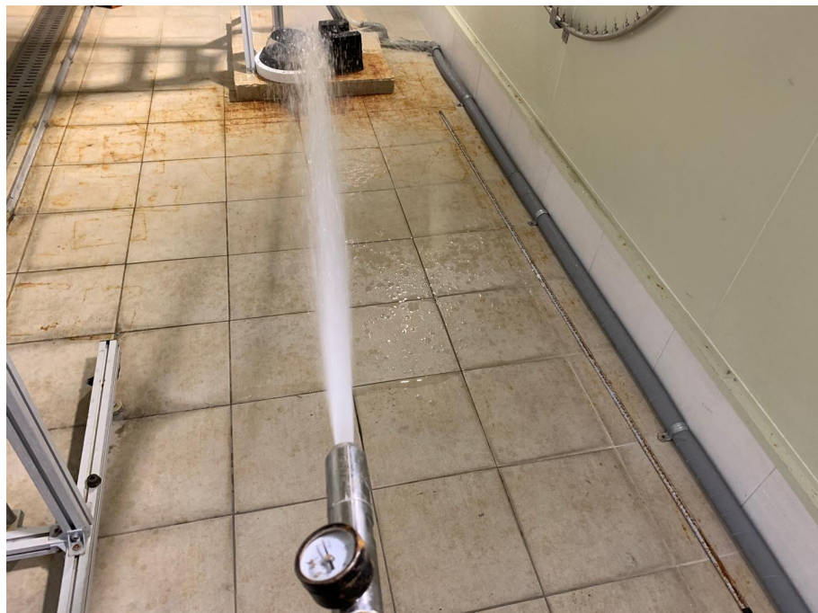
< Photo 4 > The second characteristic numeral test
