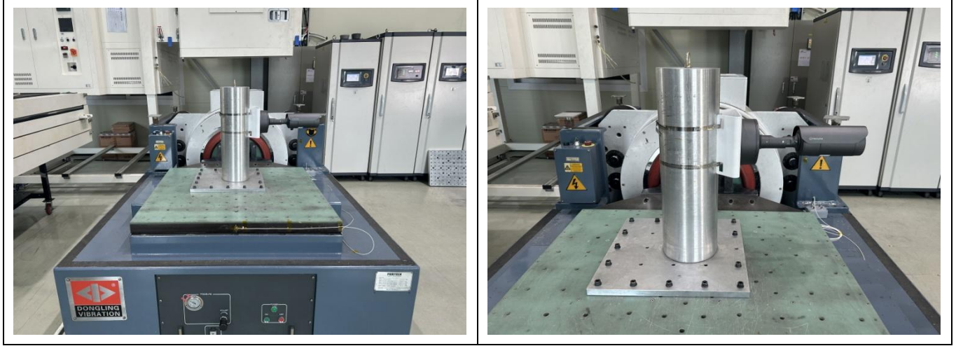
[Picture 3. Transverse (Y-axis)_set-up]
