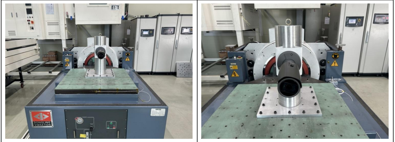
[Picture 2. Longitudinal (X-axis)_set-up]
