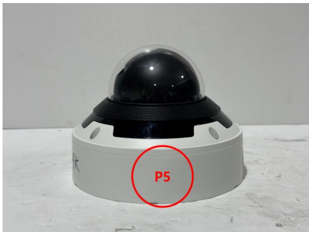
Check the hit area the test_5
