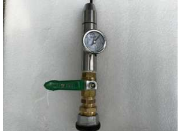
Waterproof test apparatus (IPX6)
