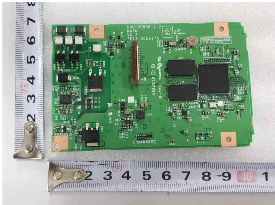
<Photo 6> Main (Power) board 후면
