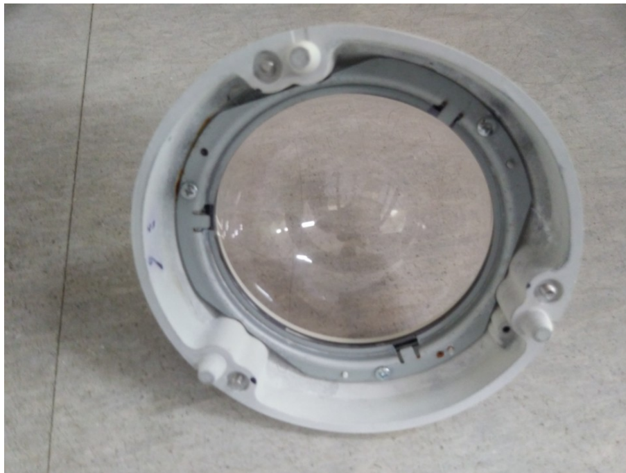
< Photo 7 > The second characteristic numeral test
