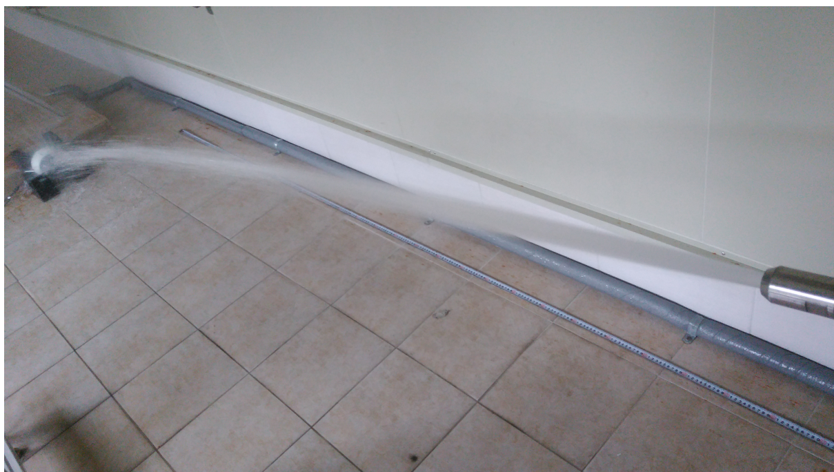
< Photo 4 > The second characteristic numeral test
