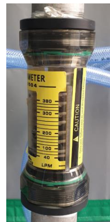
Water flow meter
