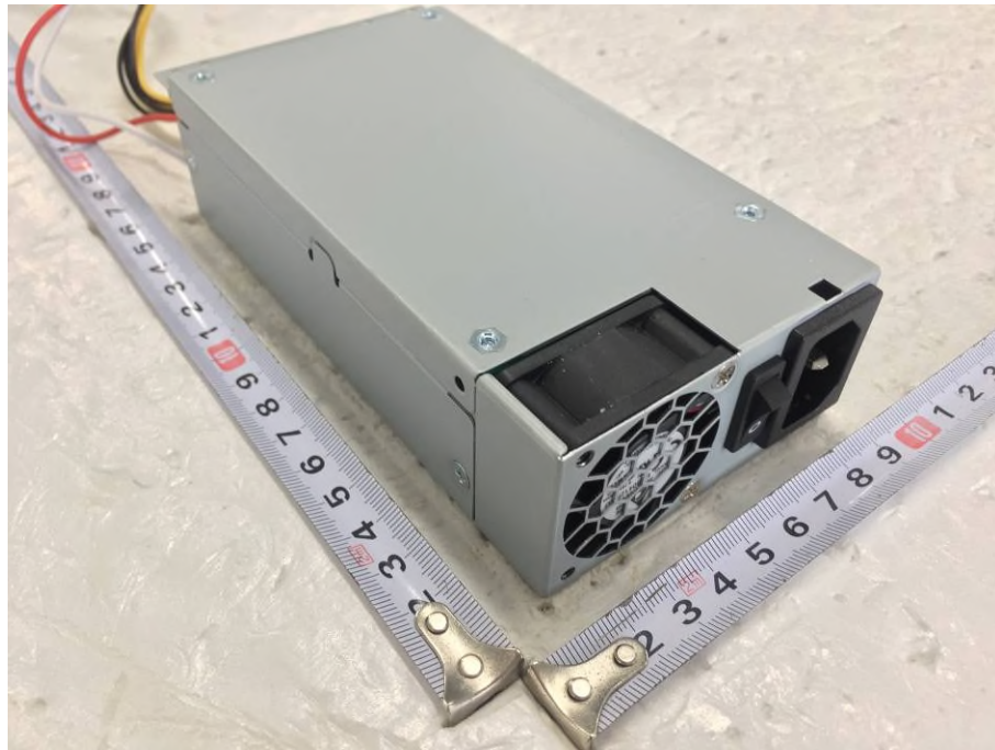
<Photo 9 > SMPS External view 2
