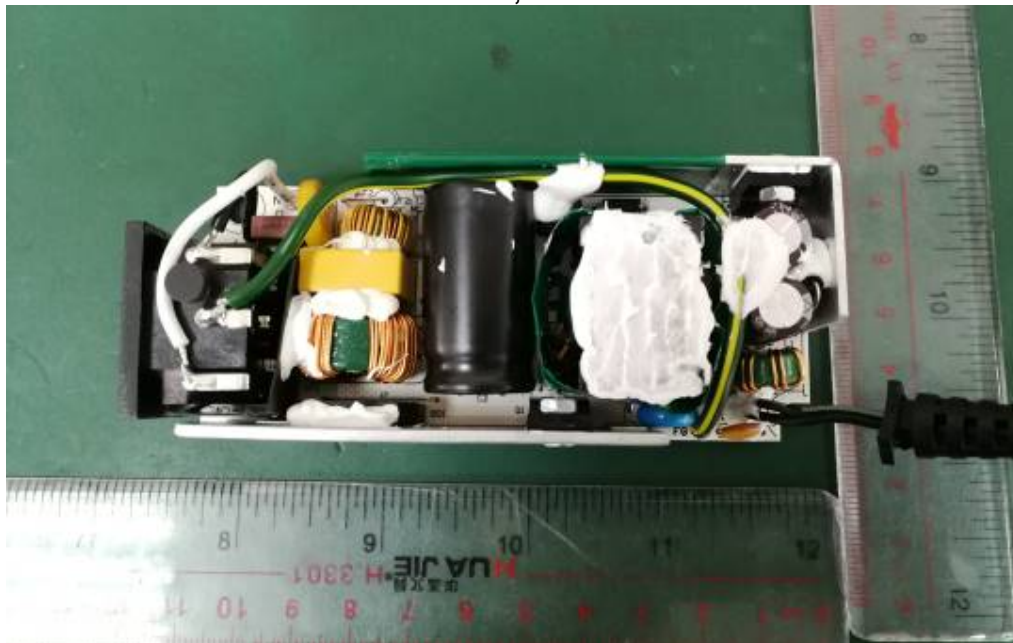
2ACL (except Y=B) Alternative PCB with R2A, R4A, F3, L1
