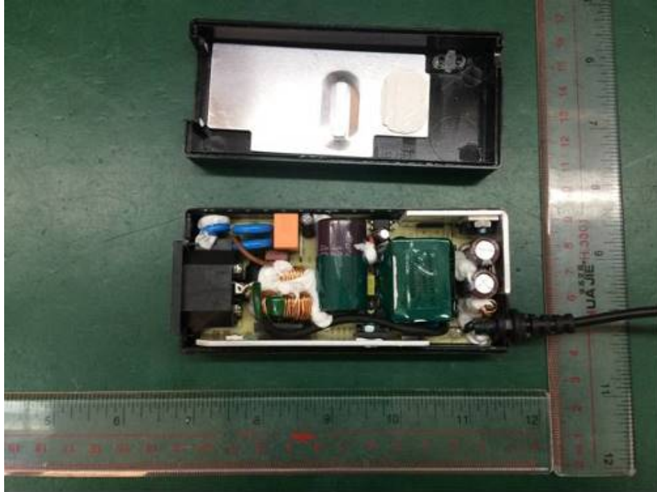
KPL: For PCB with fuses: F1 and F2 (with TVS2, TVS3, TVS4)
