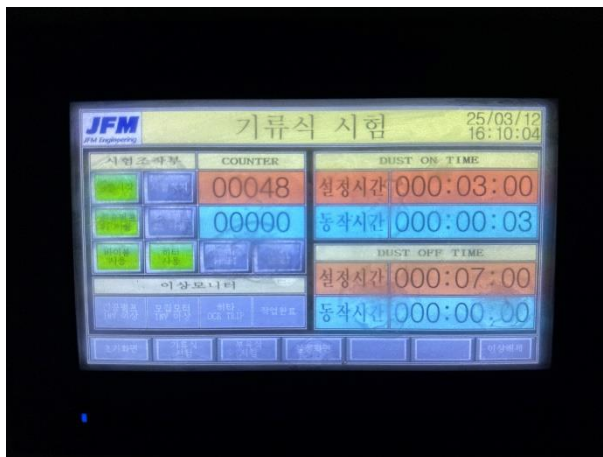
Dust test Monitor
