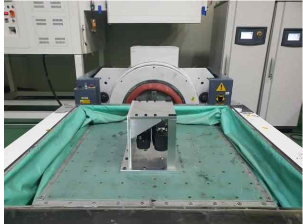
Vibration(Sine) Test[IEC/EN 60068-2-6:2007] – Y axis, Test Shock(impact) Test Same configuration
