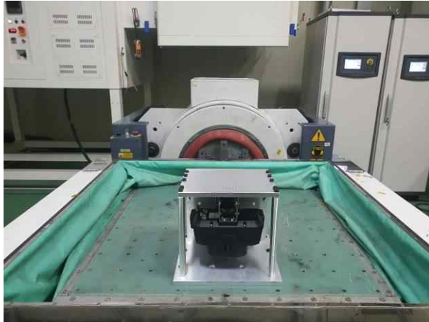
Vibration(Sine) Test[IEC/EN 60068-2-6:2007] – X axis, Test Shock(impact) Test Same configuration
