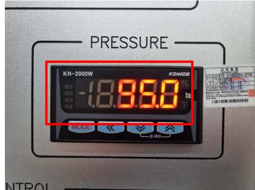
Fig. 22) Photo of the test condition (Water pressure)
