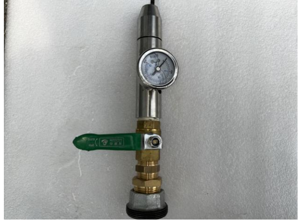
Waterproof test apparatus (IPX6)
