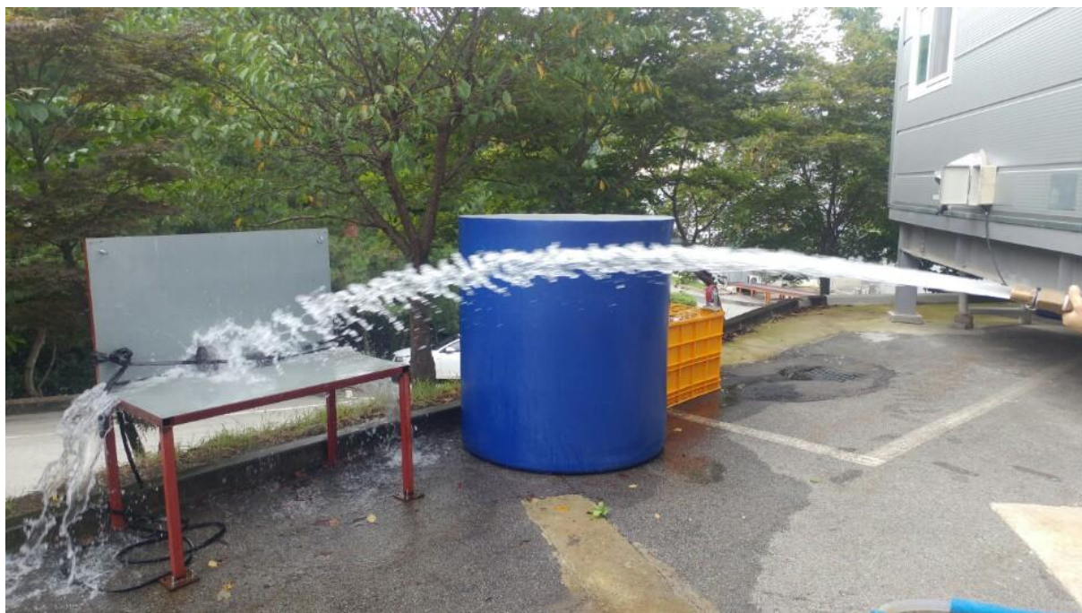
<Photo 3 > Hose down test
