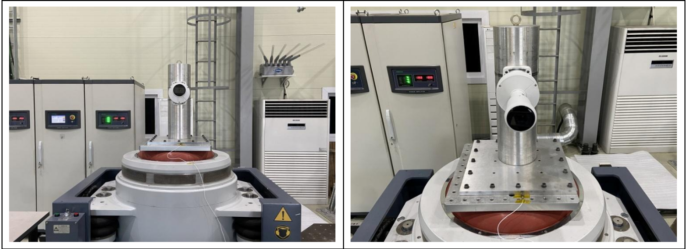
[Picture 4. Vertical (Z-axis)_set-up]
