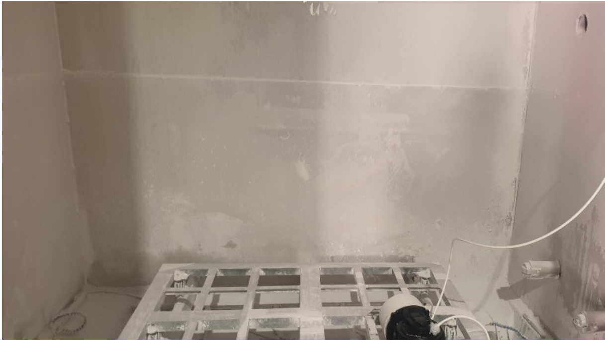
< Photo 4 > The second characteristic numeral test
