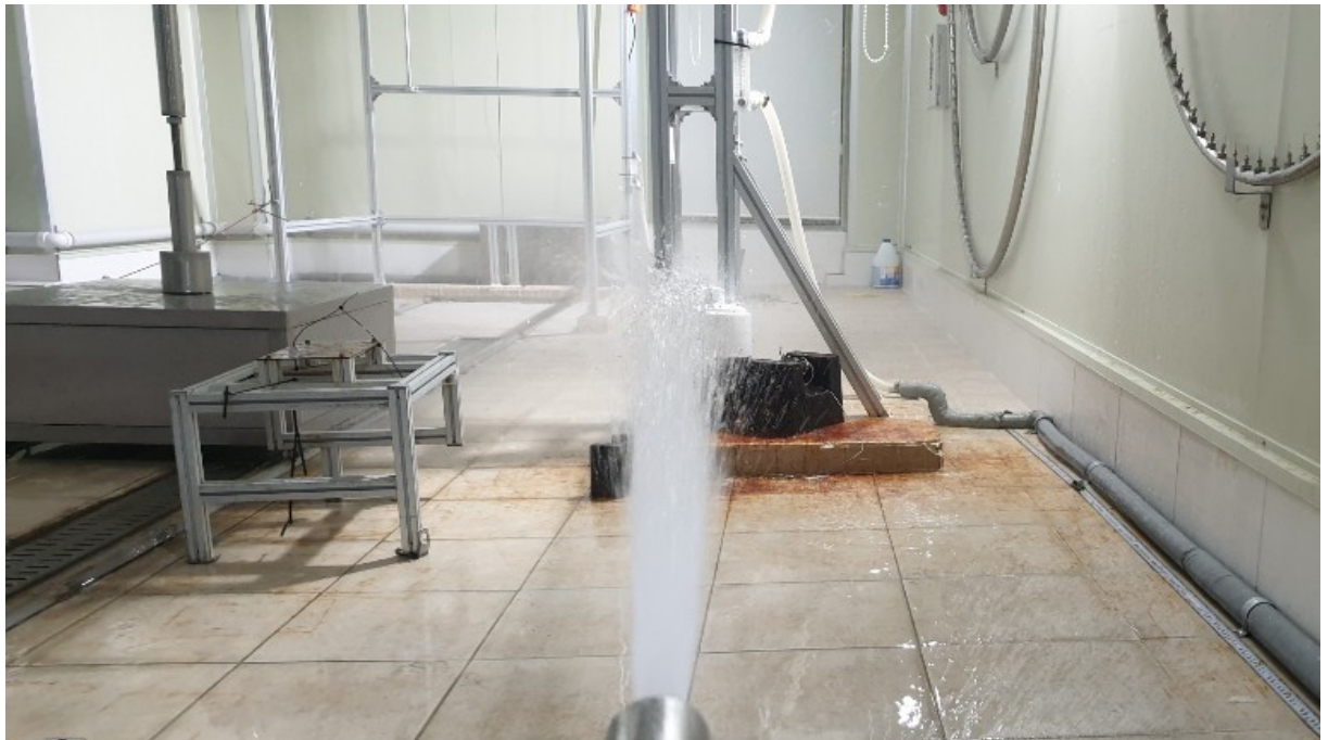
< Photo 4 > The second characteristic numeral test
