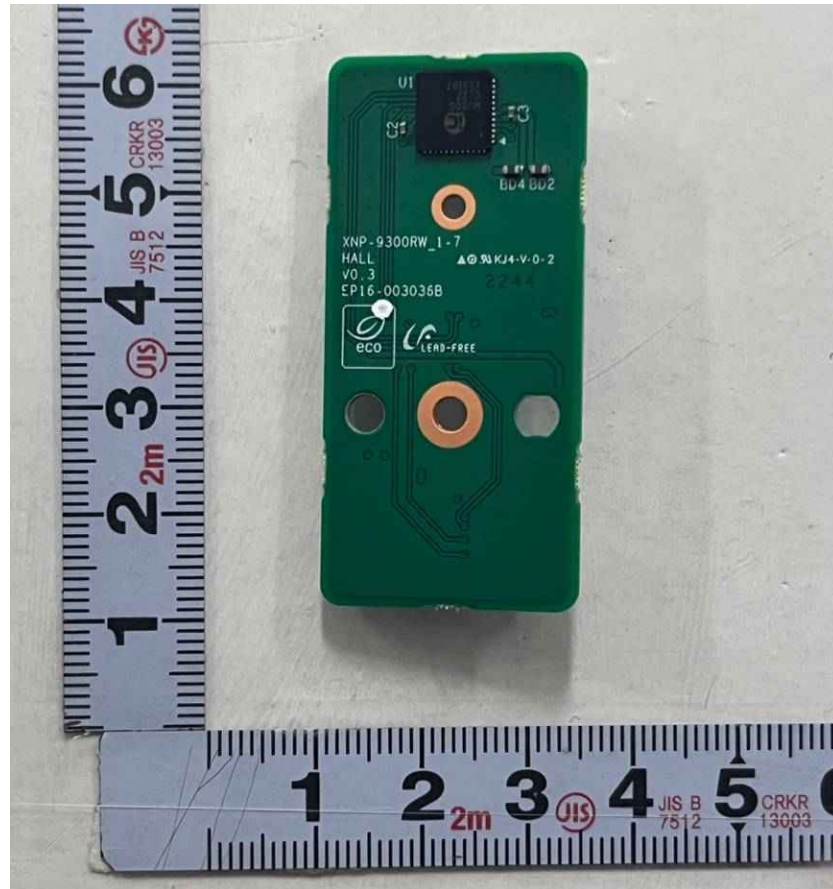
<Photo 31> Hall board bottom view
