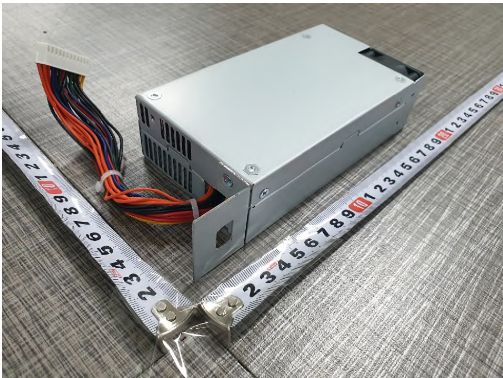
<Photo 6 > External view (SMPS)
