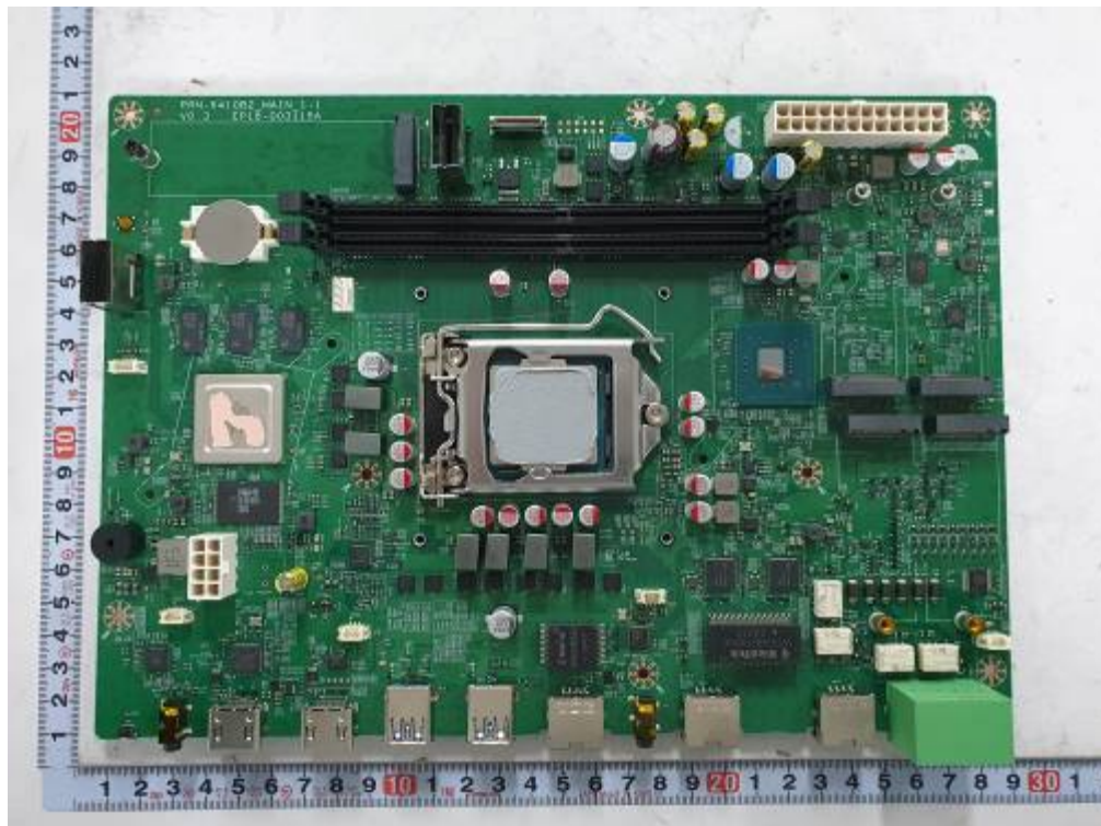
<Photo 14 > Component view (Main board - RAID type)
