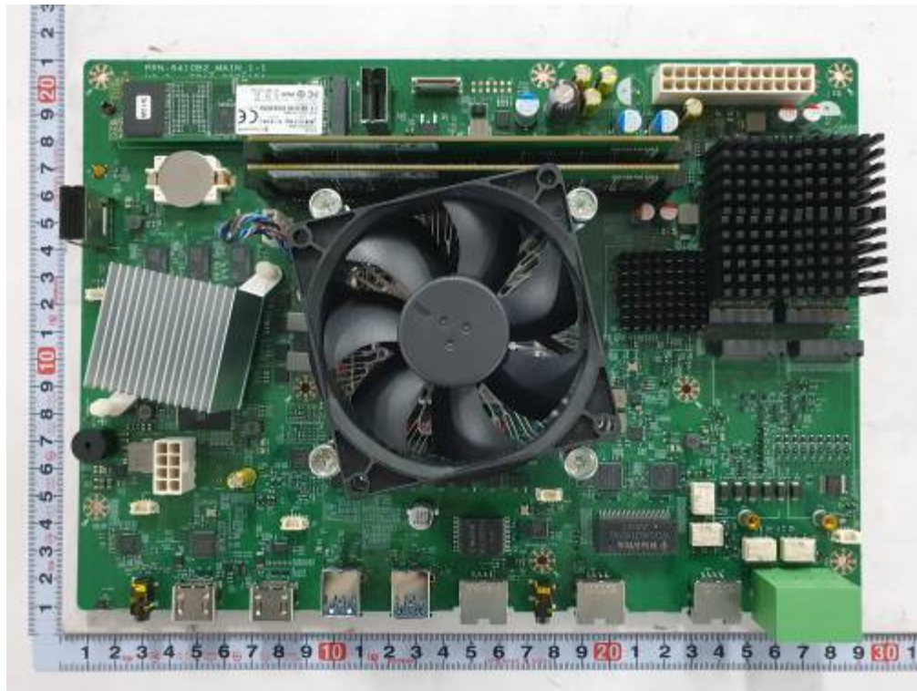
<Photo 13 > Component view (Main board - RAID type)
