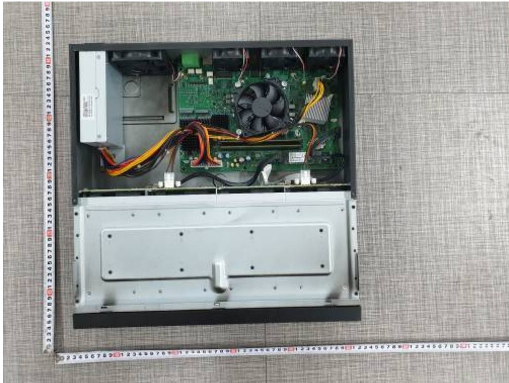
<Photo 7 > Internal view (HDD - Slot type)
