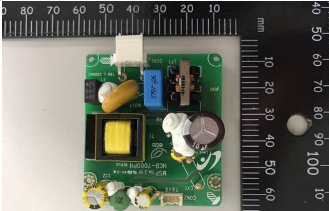
<Power supply unit internal circuit's board _ top view>
