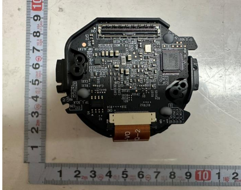
<Photo 11> Sensor board view
