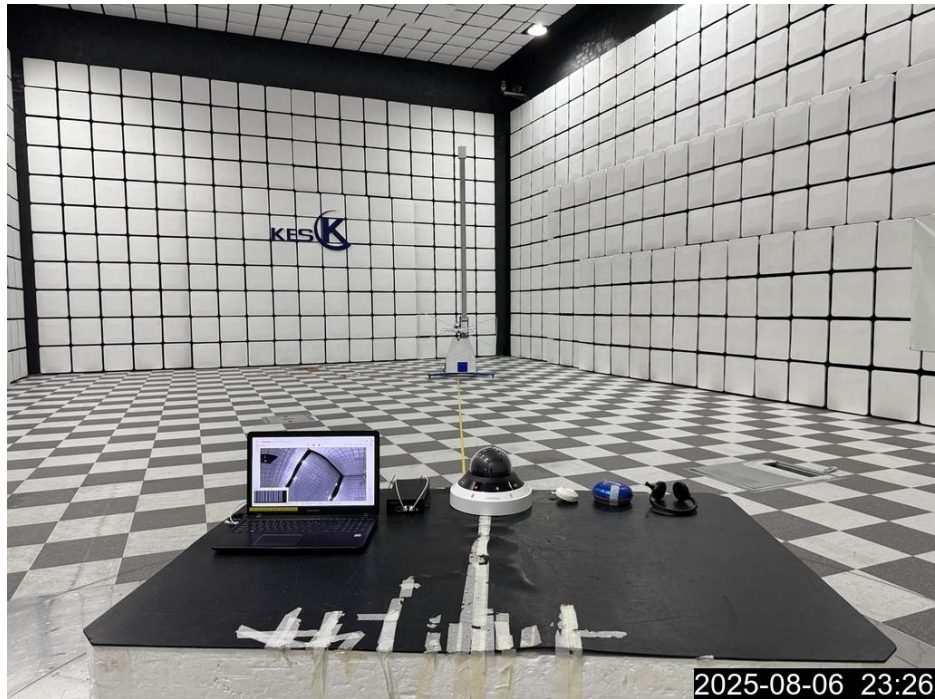
<Radiated Emissions(Below 1 GHz) - Front> Mode 2
