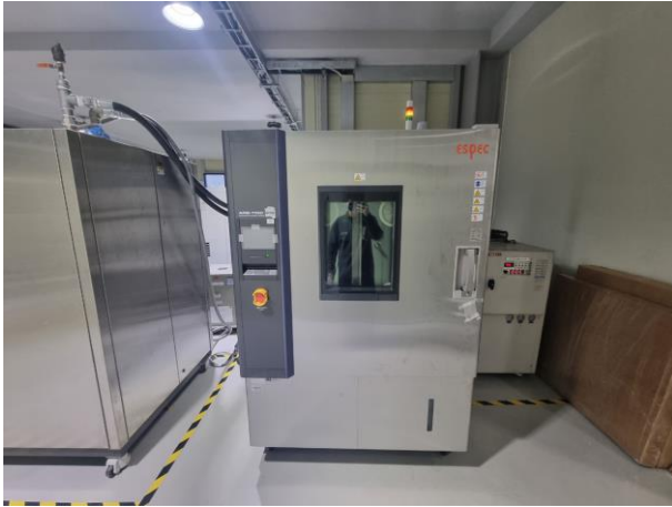
Temperature & Humidity Chamber
