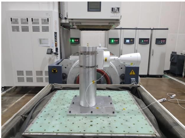
Resonant search - Y axis, Endurance, Test Shock(impact) Test Same configuration
