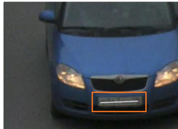
Improper focus settings. Adjust the lens.
