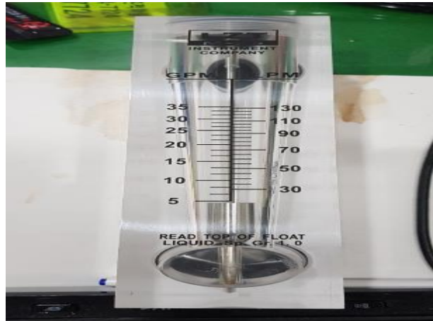
Water flow meter with IPX6
