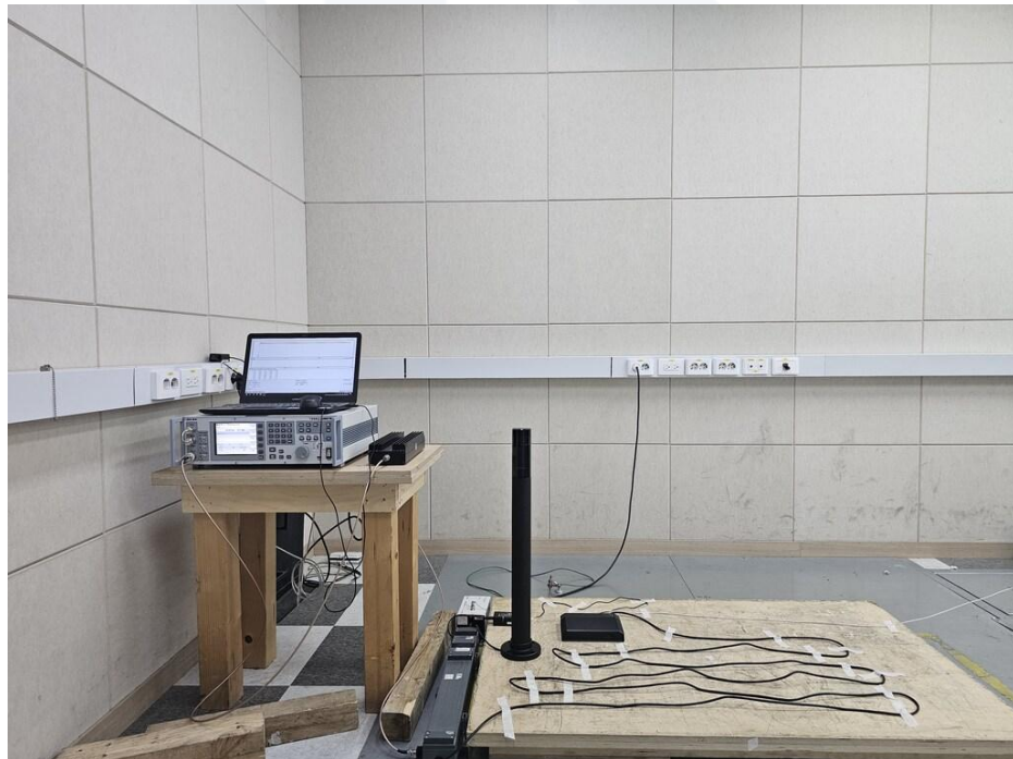
<Continuous Induced RF Disturbances>
