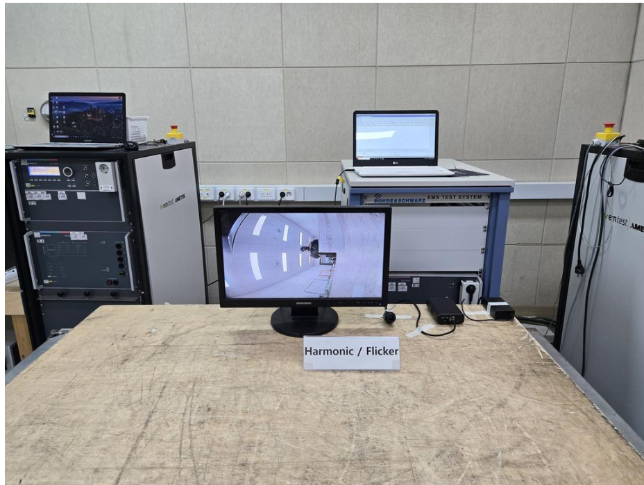
<Harmonic Current Emissions and Voltage Fluctuations and Flicker>
