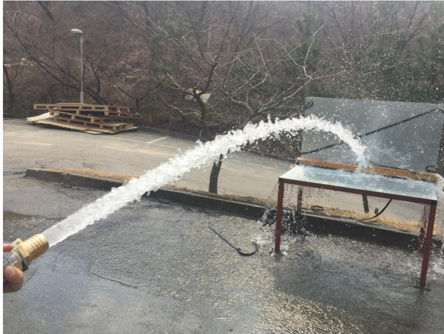
<Photo 3 > Hose down test
