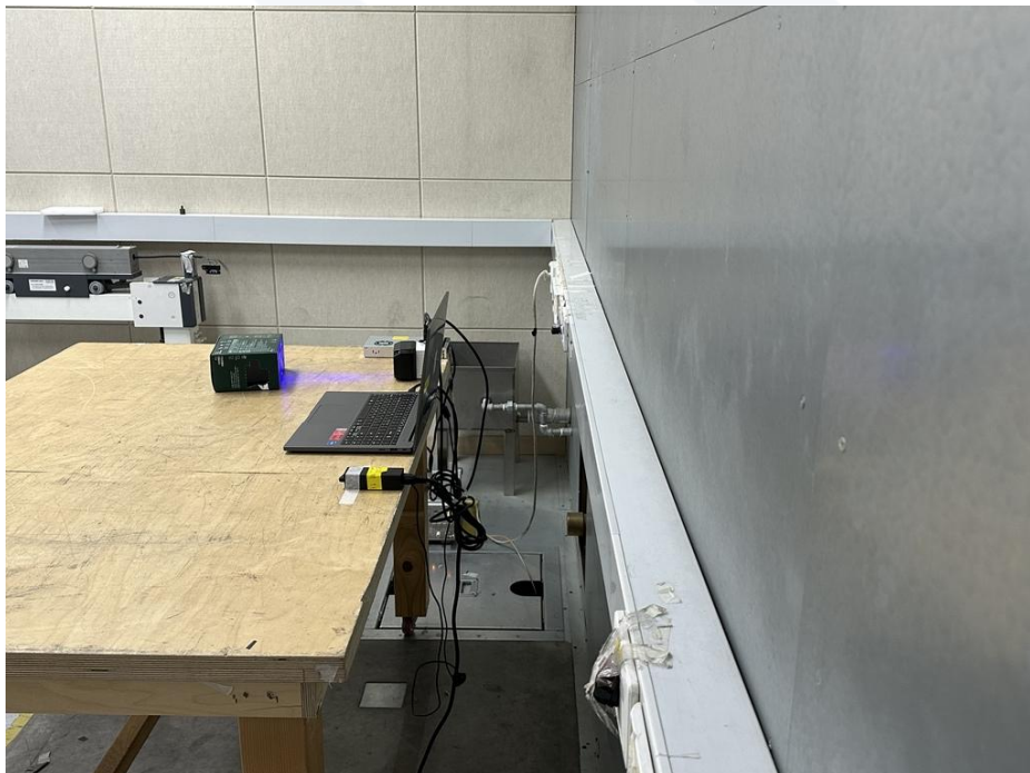
<Conducted Emissions at Mains Power Ports - Rear>
