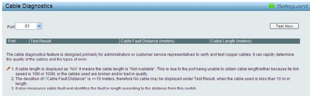
Figure 4.93 – Monitoring &gt; Cable Diagnostic
