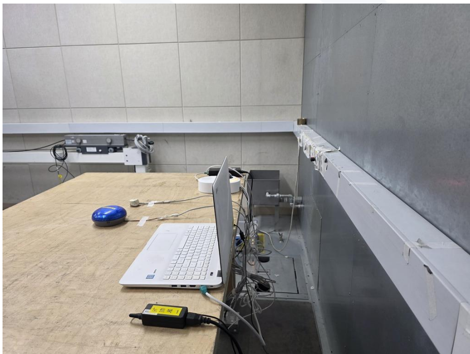
<Conducted Emissions at Telecommunication Ports - Rear>
