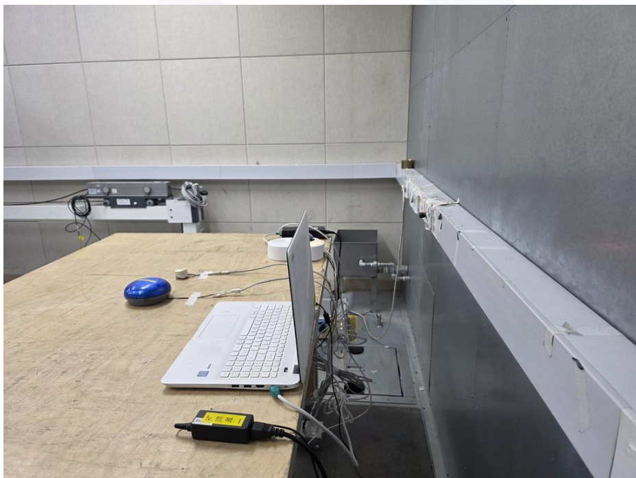
<Conducted Emissions at Telecommunication Ports - Rear>
