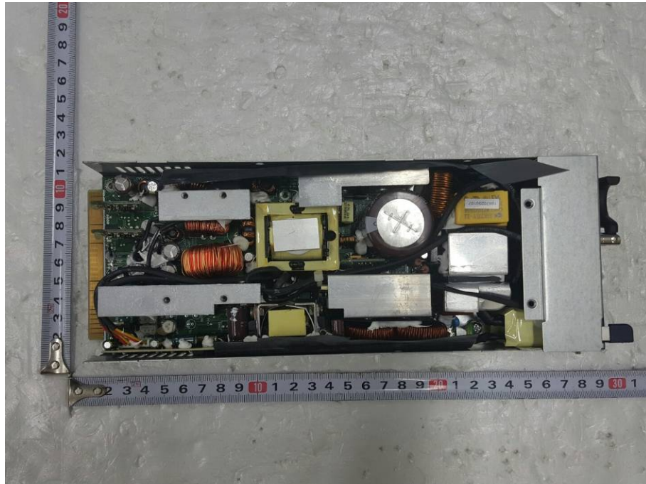
<Photo 21 > SMPS1 and SMPS2 internal view
