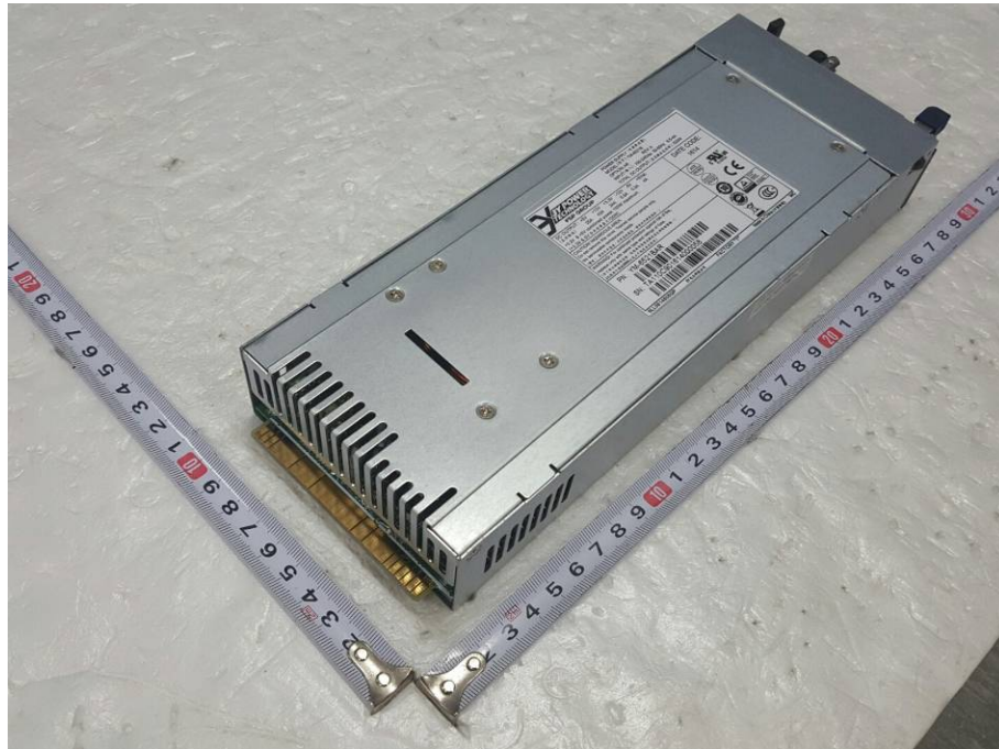
<Photo 19 > SMPS1 and SMPS2 external view 1
