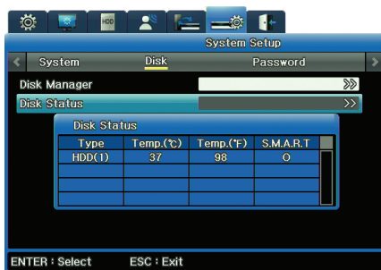
Figure 6.2.3 Disk Status submenu on the System Setup Menu
