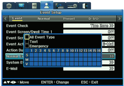
Figure 8.2.3 Normal Event Source submenu on the Event Submenu
