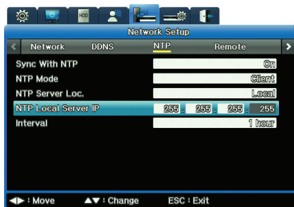
Figure 7.3.1 NTP submenu on the Network Setup Menu
