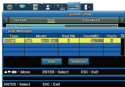
Figure 3.6.8 Disk Manager Menu Showing Enabled Hard Disk Drive
