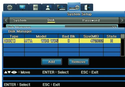
Figure 3.6.7 Disk Manager Menu Showing Disabled Hard Disk Drive
