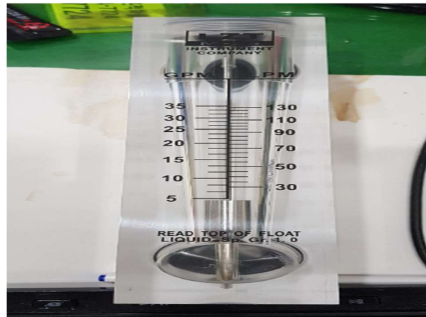
Water flow meter with IPX6
