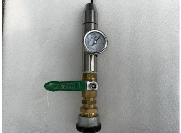
Waterproof test apparatus (IPX6)
