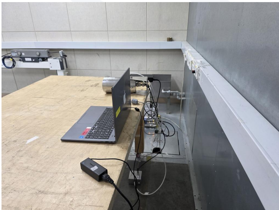
<Conducted Emissions at Telecommunication Ports - Rear>
