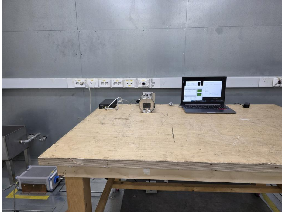
<Conducted Emissions at Telecommunication Ports - Front>
