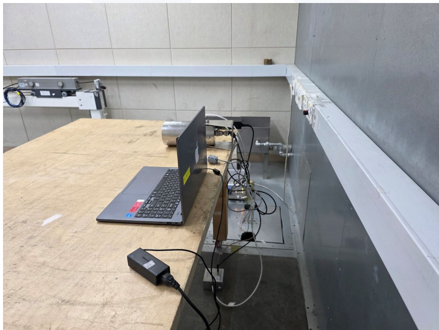
<Conducted Emissions at Telecommunication Ports - Rear>
