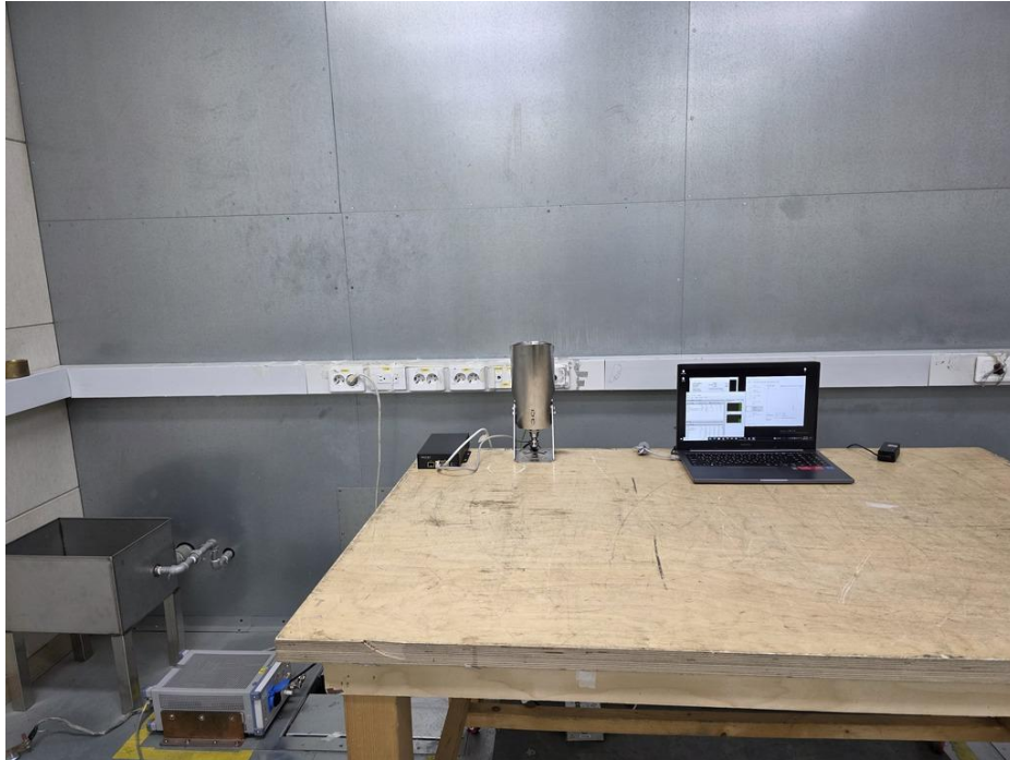
<Conducted Emissions at Telecommunication Ports - Front>
