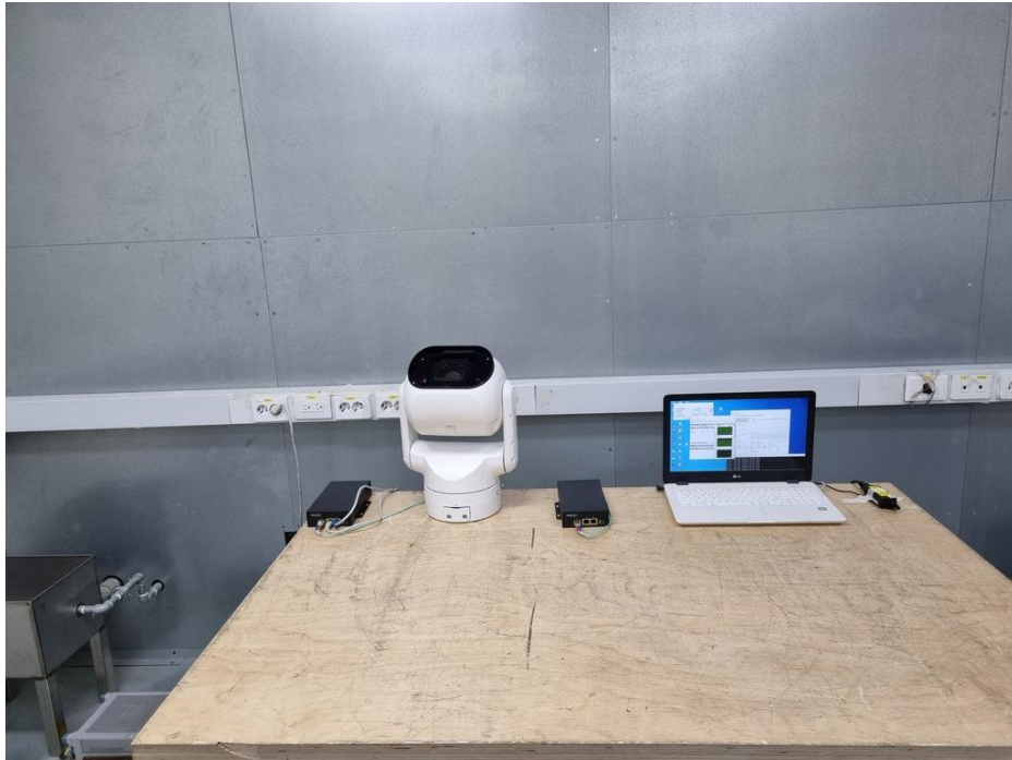
<Conducted Emissions at Telecommunication Ports - Front>
