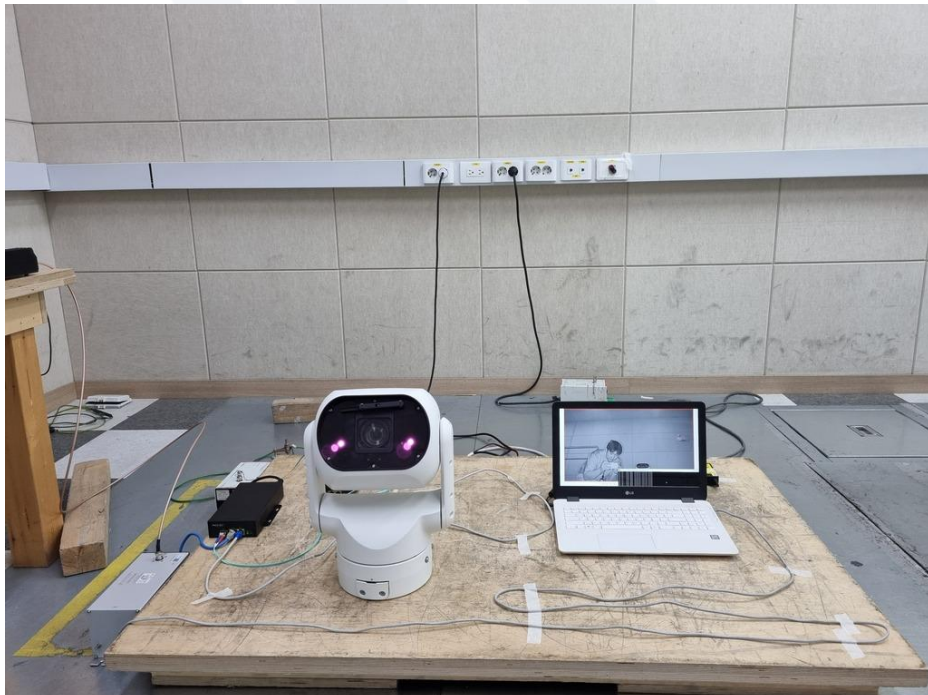
<Continuous Induced RF Disturbances>
