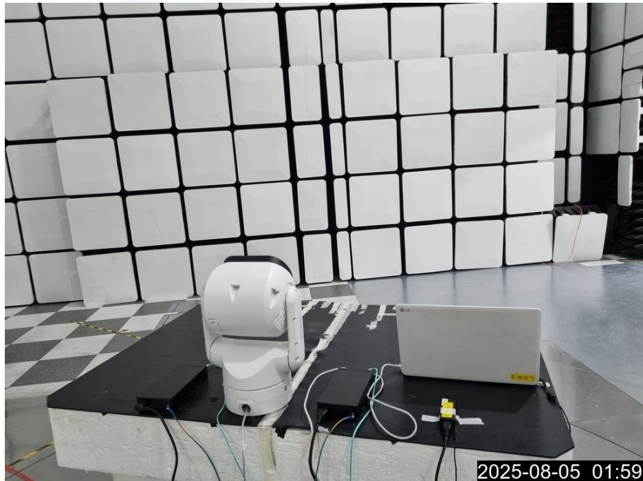
<Radiated Emissions(Below 1 GHz) - Rear>
