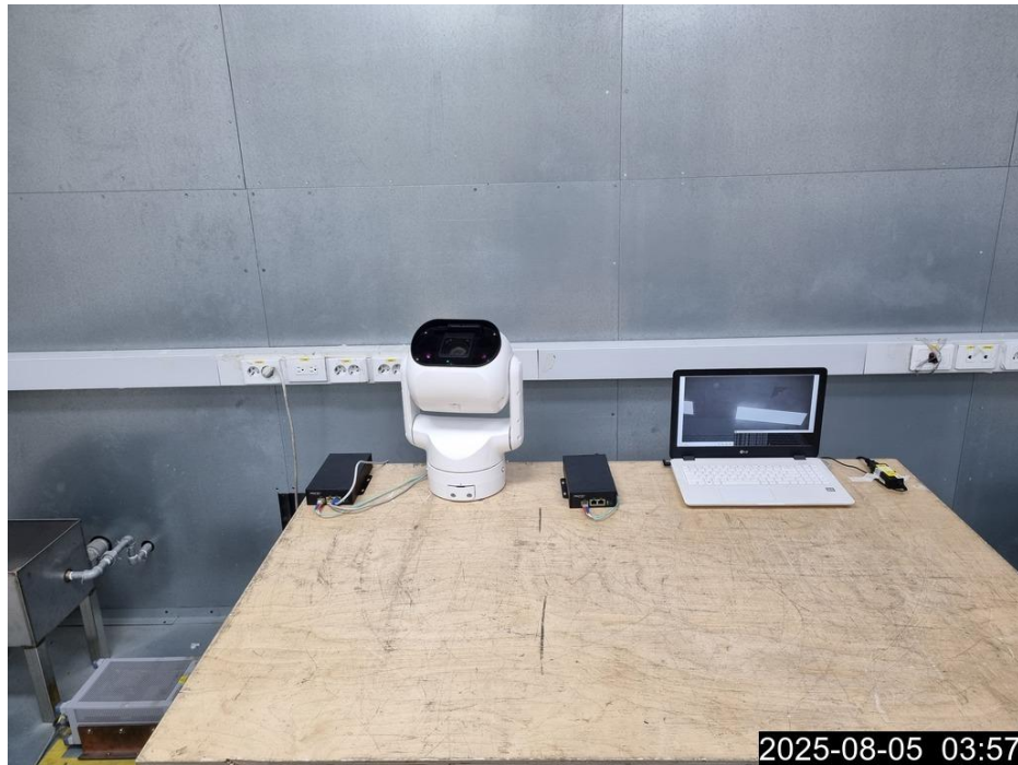
<Conducted Emissions at Mains Power Ports - Front>
