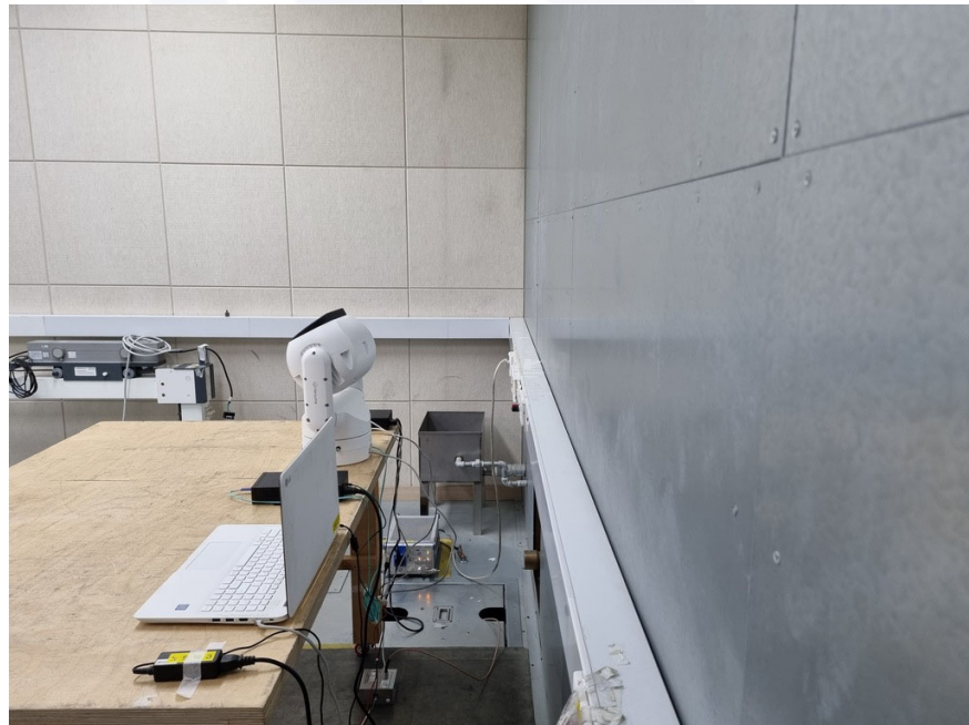
<Conducted Emissions at Telecommunication Ports - Rear>
