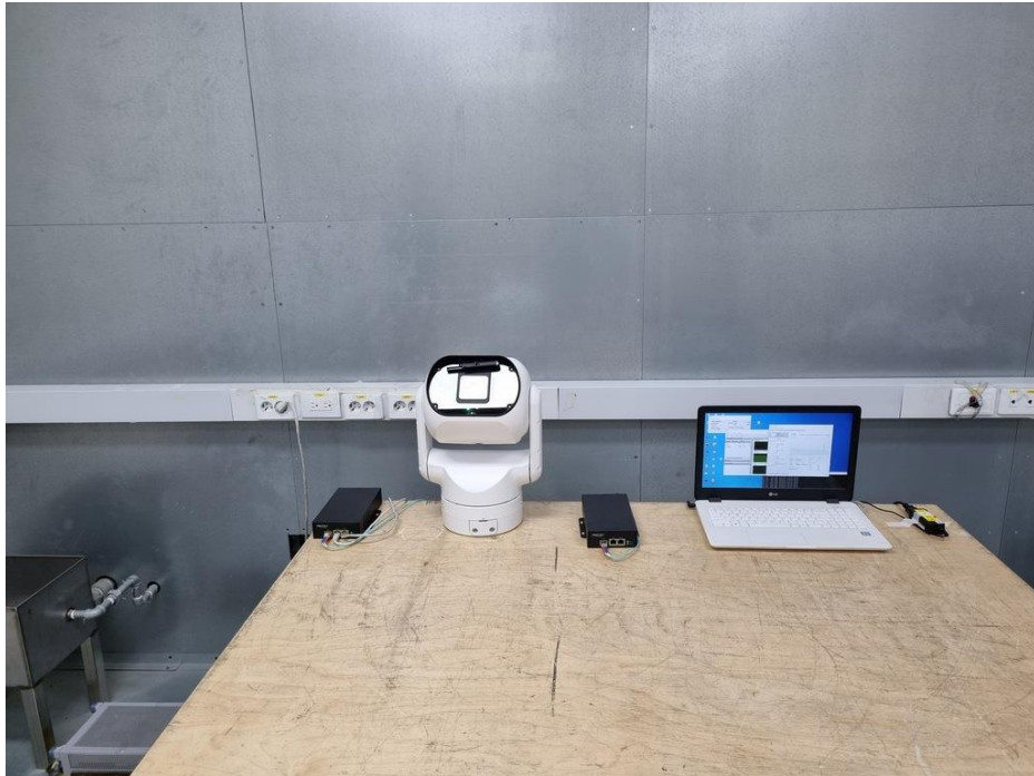
<Conducted Emissions at Telecommunication Ports - Front>
