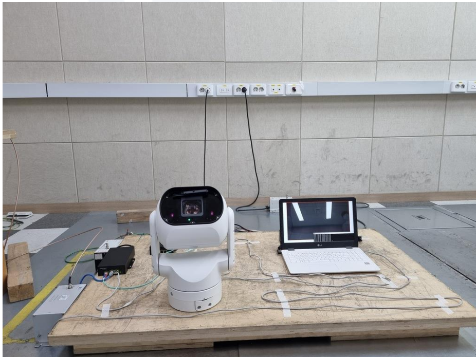
<Continuous Induced RF Disturbances>
