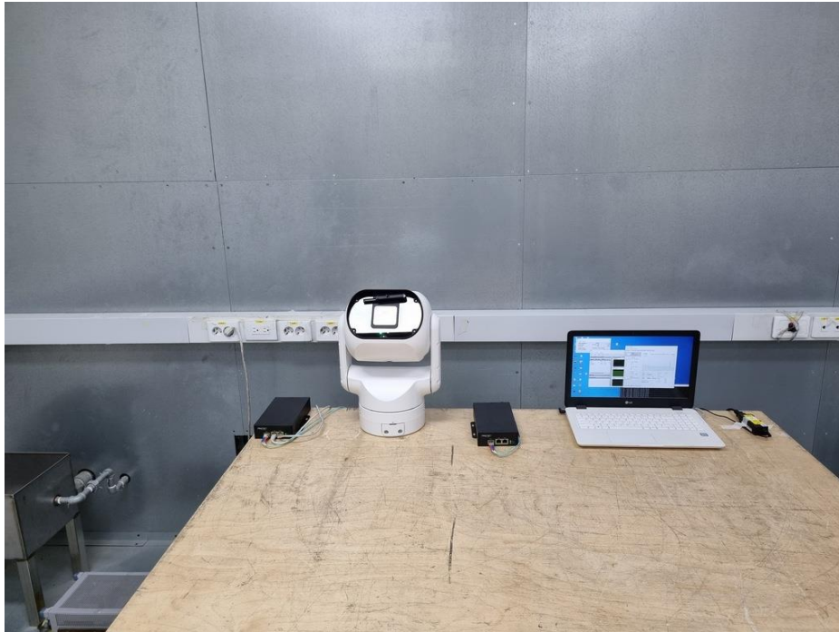
<Conducted Emissions at Telecommunication Ports - Front>
