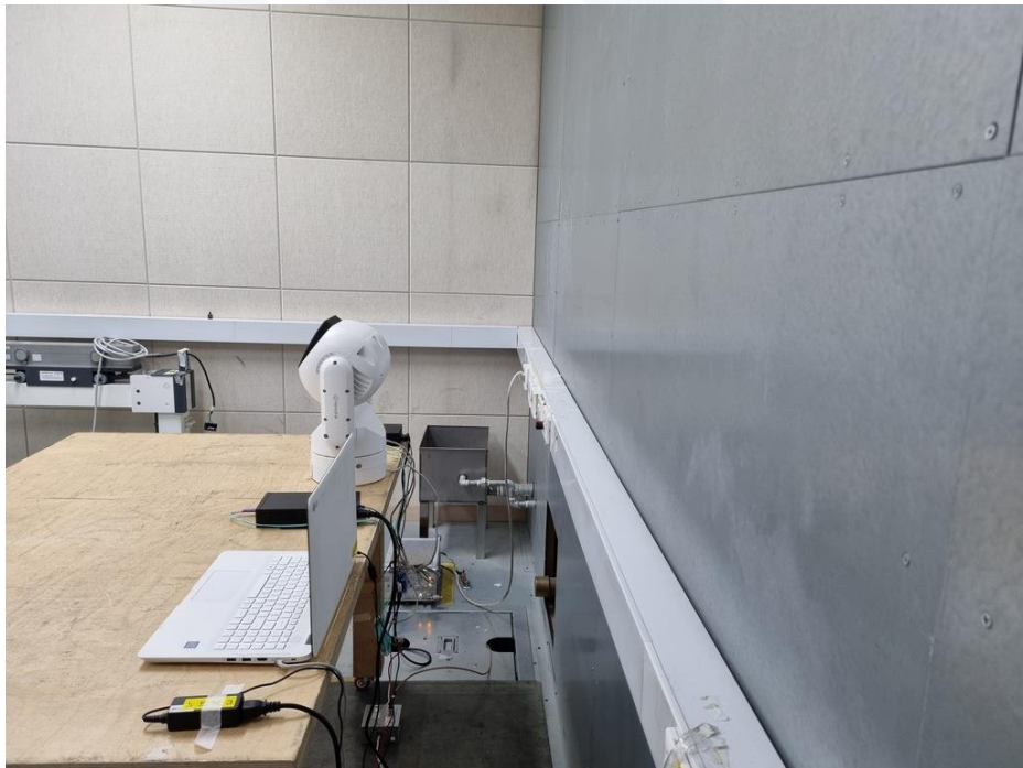
<Conducted Emissions at Telecommunication Ports - Rear>
